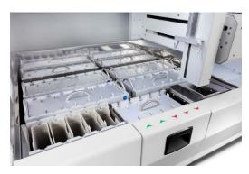
The agitation of the reagent dishes is particular and innovative, it is completely independent from the automatic arm. This particular agitation system (called "WAVING") allows to obtain omogeneity of the staining solutioninside the dish, improving the quality of section staining and, last but not least, it reduces the amount of precipitate produced during daily routine.
