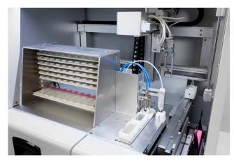
Unique and exclusive exit system of mounted glass slides: Bio-optica instrument ALLOWS TO OBTAIN THE MOUNTED GLASS SLIDES DIRECTLY ON TRAYS IN HORIZONTAL POSITION, by avoiding a huge time waste for the operators who will be able to bring the trays directly to the pathologist for the evaluation at the microscope.
